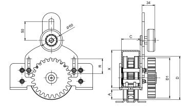
Movement is generated by the ground mounted rack that also functions as a track.
