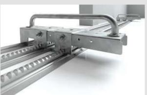
The Rack Track installation templates are used to ensure a precise and parallel alignment of the tracks and rack tracks, and can be width regulated depending on the thickness of the tubular profile used in the construction of the gate.
